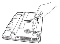
(Sample Illustration) Unlocking the battery release lock
